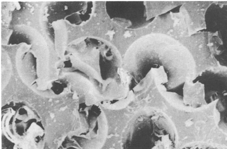
Figure 6 Crushed cells of foamed polyurethane.
